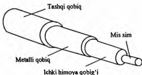
6.2-rasm. Koaksial kabel tuzilishi.
