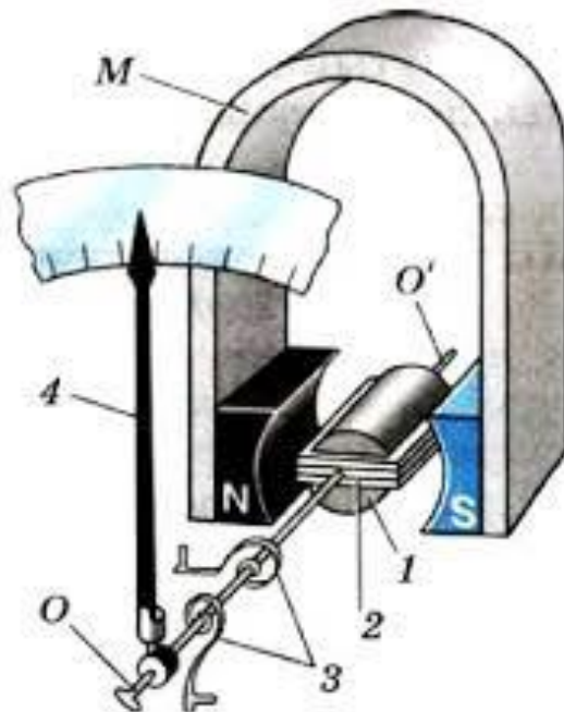
4.1-rasm. Magnitoelektrik asbobning tuzilishi. 1-doimiy magnit, 2-harakatchan g'altak (ramka), 3-spiralsimon prujina, 4-strelka, o'zak.
